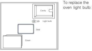
1. Remove the glass cover using a screwdriver. 2. Unscrew the light bulb and replace it with a similar one: Wattage 15 W, cap E 14. Replace the glass cover, making sure the seal is positioned correctly (*see diagram*).
